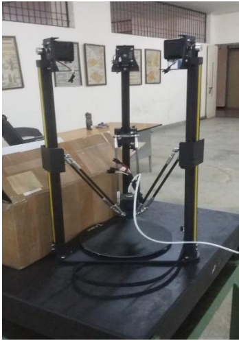
Fig 19: Semi Assembled Delta 3D-printer
